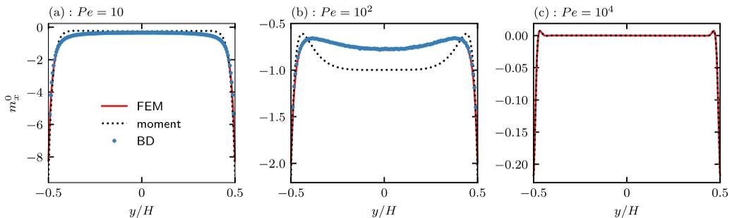
FIG. 10. The average polar order distribution ( $m_x^0$ ) across the channel for different Péclet numbers ( $Pe = u_0 H / D_T$ ) with  $\ell/H = U_0 \tau_R / H = 10$  and  $\ell/\delta = U_0 \tau_R / \sqrt{D_T \tau_R} = 30$ . The red solid lines are solutions from FEM, the black dashed lines are from moment equations, and the blue dots are results from BD simulation.
