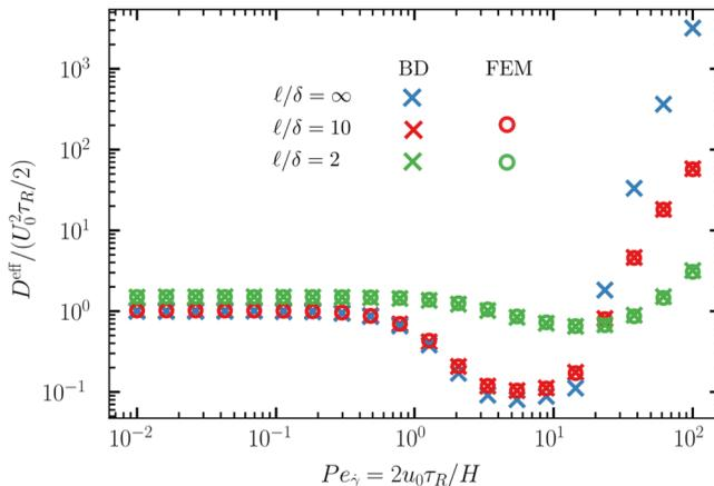
FIG. 14. The effective longitudinal dispersion coefficient  $D^{\text{eff}}/(U_0^2 \tau_R/2)$  as a function of  $Pe_\gamma$  for different values of  $\ell/\delta$ . The degree of confinement is fixed,  $\ell/H = 2$ . For a given  $Pe_\gamma$  and  $\ell/H$ , decreasing  $\ell/\delta$  corresponds to increasing the translational diffusivity.
