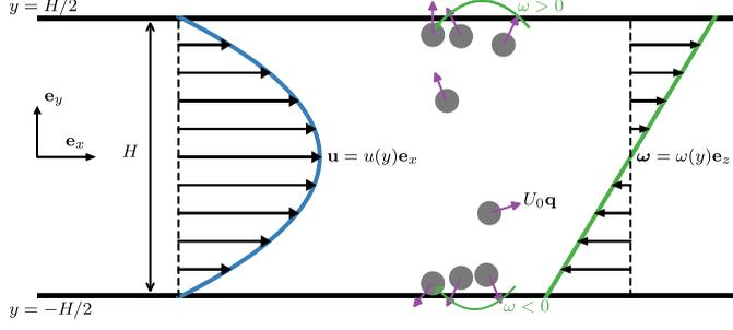
FIG. 4. Schematic of active Brownian particles suspended in a planar Poiseuille flow between two parallel plates. The ABPs reorient on a time scale of  $\tau_R = 1/D_R$ , where  $D_R$  is the rotary diffusivity. The blue solid line is the Poiseuille flow and the green solid line is the scalar vorticity. The arrows represent the magnitude and sign of the fluid speed or vorticity. The vorticity is an odd function of the transverse coordinate  $y$ .
