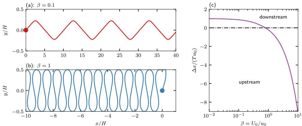
FIG. 5. (a), (b) Trajectories of a non-Brownian active particle for different speed ratios  $\beta = U_0/u_0$ . The initial positions are marked by dots. (c) Average speed in the longitudinal direction as a function of  $\beta$ . Initial conditions for all three panels are identical:  $x_0 = 0$ ,  $y_0 = 0$ ,  $\theta_0 = \pi/2$ .
