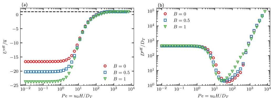
FIG. 15. (a) The average drift  $U^{\text{eff}}/\bar{u}$  as a function of  $Pe$  for different values of  $B$ . The black dashed line is the result for passive Brownian particles,  $U^{\text{eff}}/\bar{u} \equiv 1$ . (b) The effective longitudinal dispersion coefficient  $D^{\text{eff}}/D_T$  as a function of  $Pe$  for different values of  $B$ . In both panels,  $\ell/H = 10$  and  $\ell/\delta = 30$ . Results are obtained from FEM simulation of the Smoluchowski equation.
