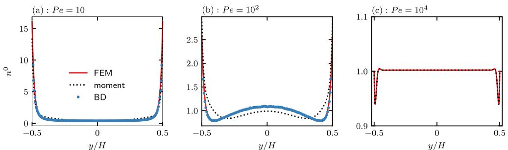
FIG. 11. The average number density distribution ( $n^0$ ) across the channel for different Péclet numbers ( $Pe = u_0 H / D_T$ ) with  $\ell/H = U_0 \tau_R / H = 10$  and  $\ell/\delta = U_0 \tau_R / \sqrt{D_T \tau_R} = 30$ . The red solid lines are solutions from FEM, the black dashed lines are from moment equations, and the blue dots are results from BD simulation.
