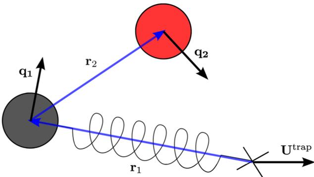
**FIG. 1.** Schematic of the pair problem of a spherical probe particle (gray) in a moving harmonic trap interacting with a spherical bath particle (red). Both the probe and the bath particles can be active.
